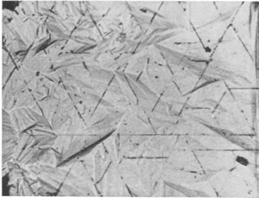
Figure 3 Microcracks in ZnS layers epitaxially grown on (\bar{1}\bar{1}\bar{1}) GaP surface (approx. \times 15 ).
